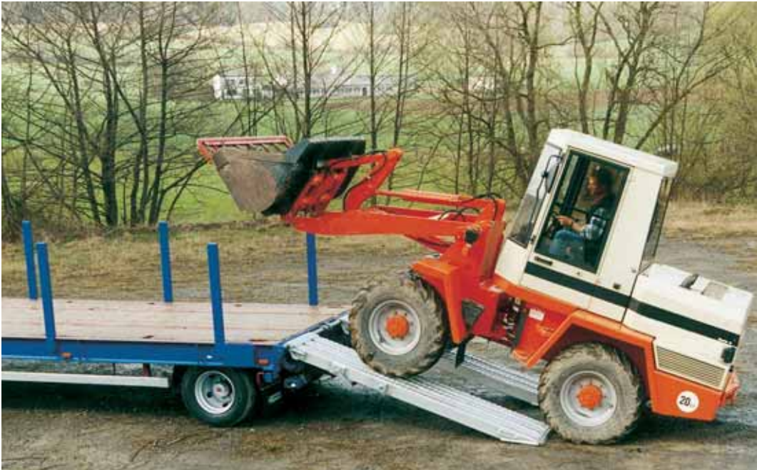
As an option, the ramps can be fitted with a spring system.
