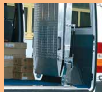
The RRD can rotate inside and outside of the vehicle
